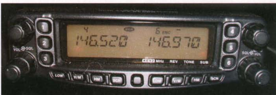
Figure 3. An example of a dual-band FM transceiver (Yaesu FT-8900) that is capable of being a crossband repeater.
