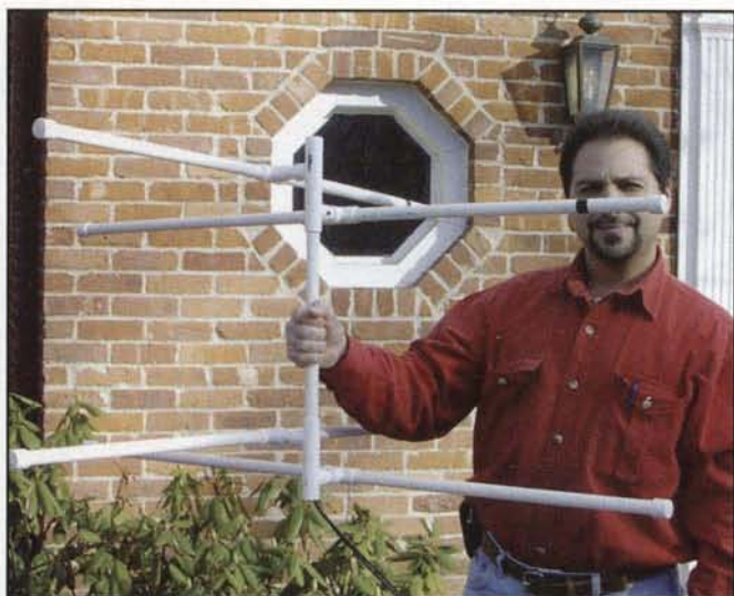
Figure 6. A simple, but effective, satellite receiving antenna can be made from materials purchased from your local home-improvement store. The antenna is unobtrusive, lightweight, and easily installed on a rooftop.
