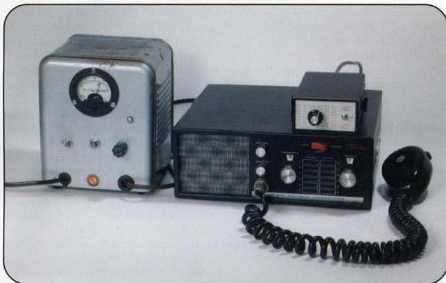
Photo C. Variable-voltage power supply built from components of an old battery booster, powering a vintage Regency HR-212 two-meter FM rig. A CTCSS access tone encoder sits atop the rig.
